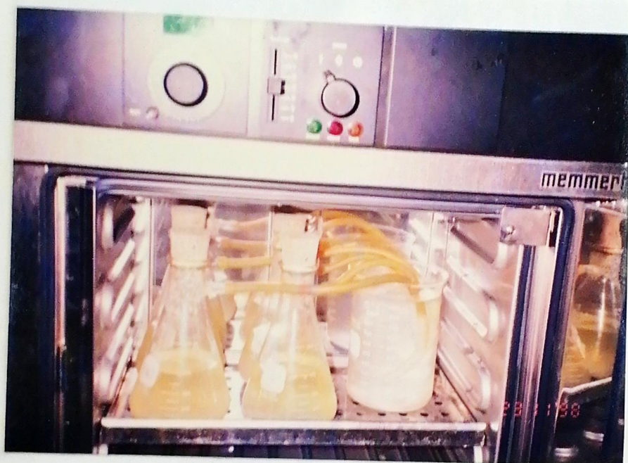
Plate 3.0 The Fermentation set-up at 35^{\circ}\text{C} – 42^{\circ}\text{C} for 7 days.
