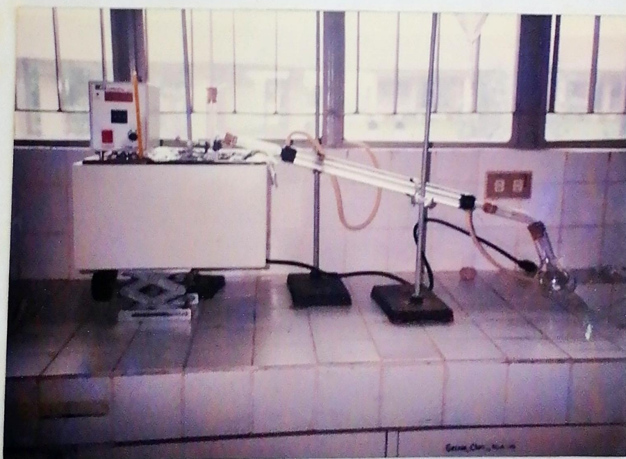
Plate 4.0 The distillation set-up using the constant temperature water-bath for temperature control.
