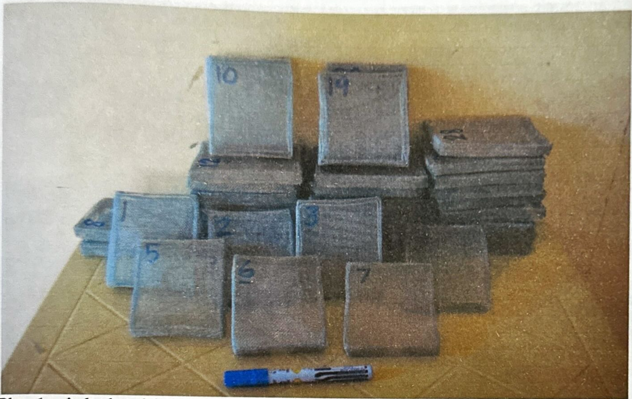
Plate 1. wirebaskets labeled and used for water stability test.
