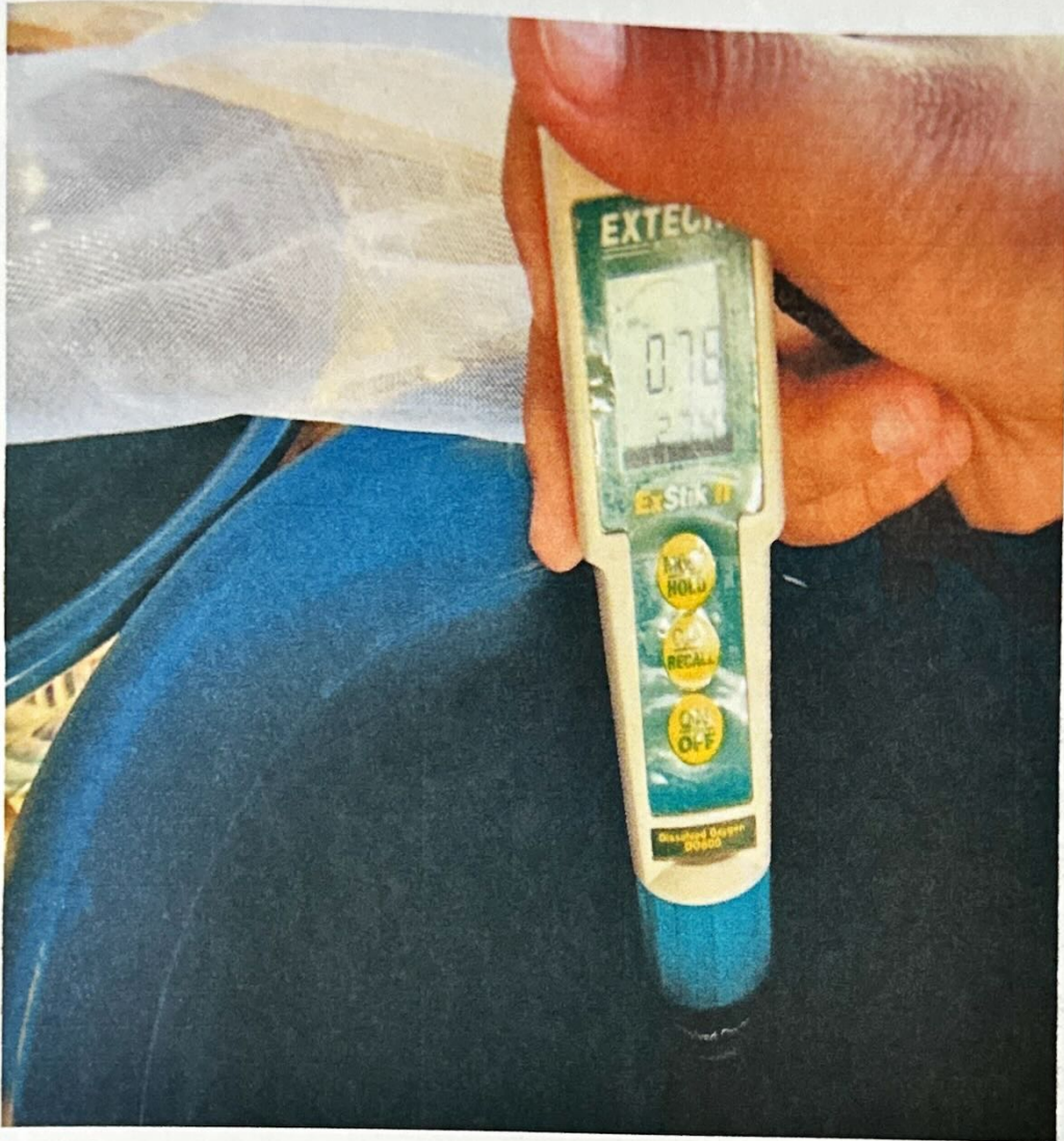
Plate 6. Measuring the dissolved Oxygen and Temperature of water samples
