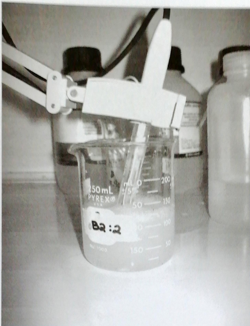
Plate 2. Determination of pH using a pH meter
