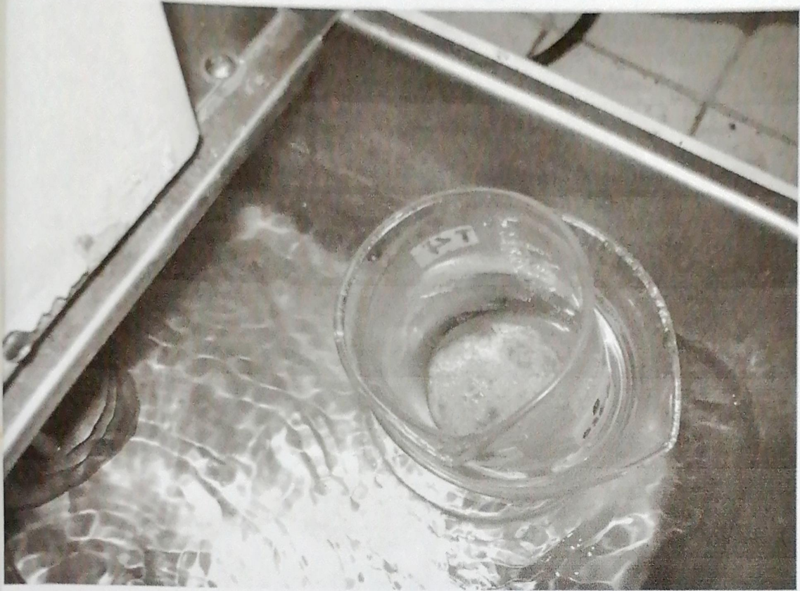
Plate 3. Liberation of fatty matter using 2M \text{H}_2\text{SO}_4
