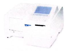
The spectrophotometer model UV mini-1240 Shimadzu at the South East Asian Fisheries and Development Center (SEAFDEC) was used in the study. Its wavelength range is from 190.0 ~
