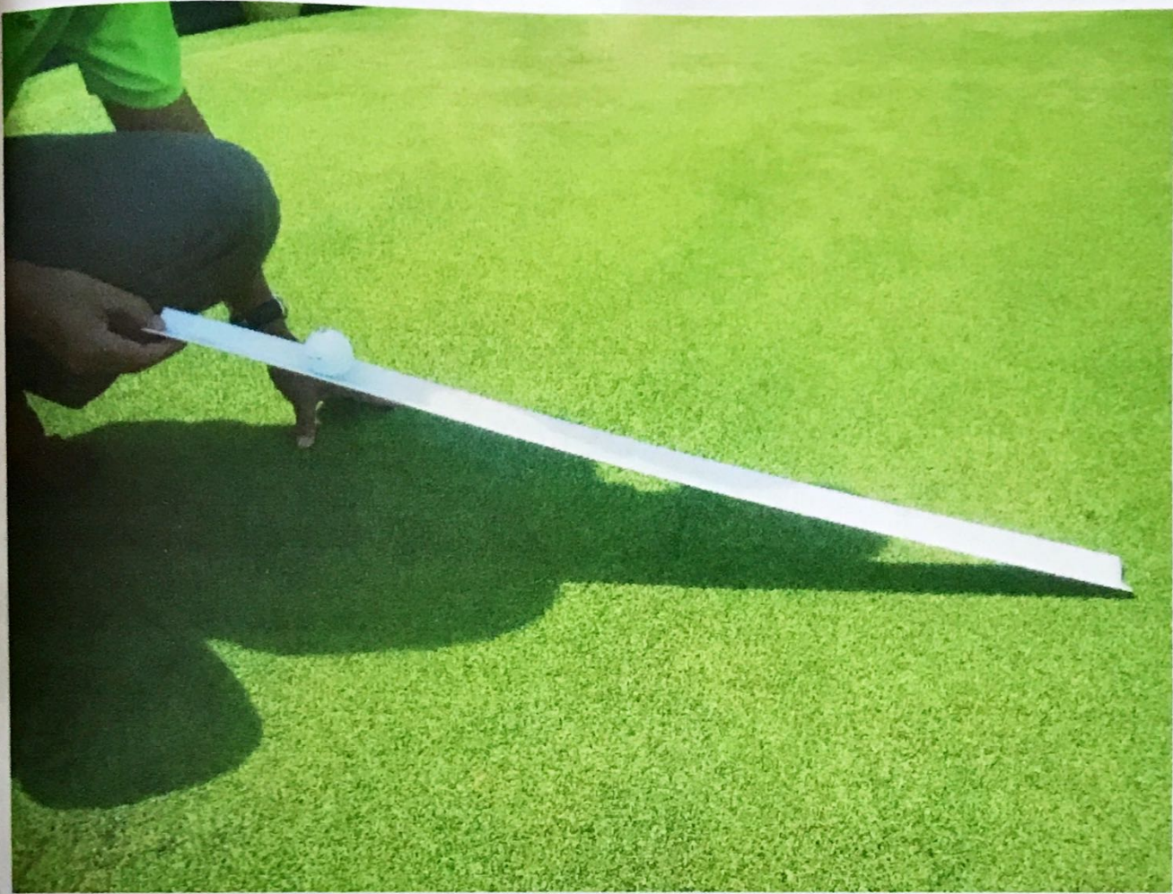
Figure 4. Releasing the Golf Ball with the Stimpmeter
